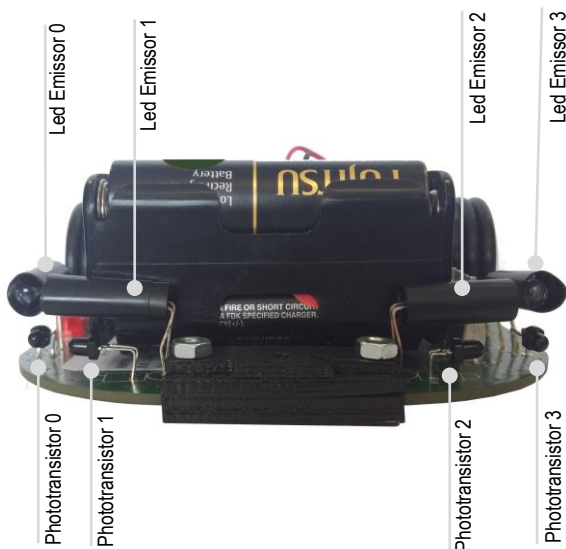
Img 34 Identification of phototransistors and emitter LEDs
